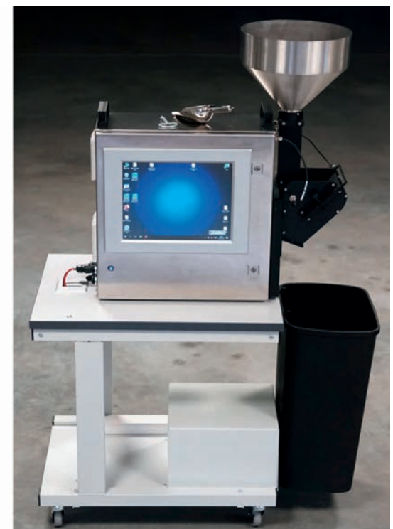
Fig. 4. The two laboratory instruments Spectro-T-3-DIF/0°-Lab-CMU and Spectro-T-3-DIF/0°-Mobile-P are based on the same technology and are also suitable for calibrating the inline sensors.
